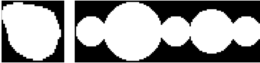
Figure 6. Two inlet geometries: a cross section of an abnormal vessel (left) and a row of intersecting circles (right).
